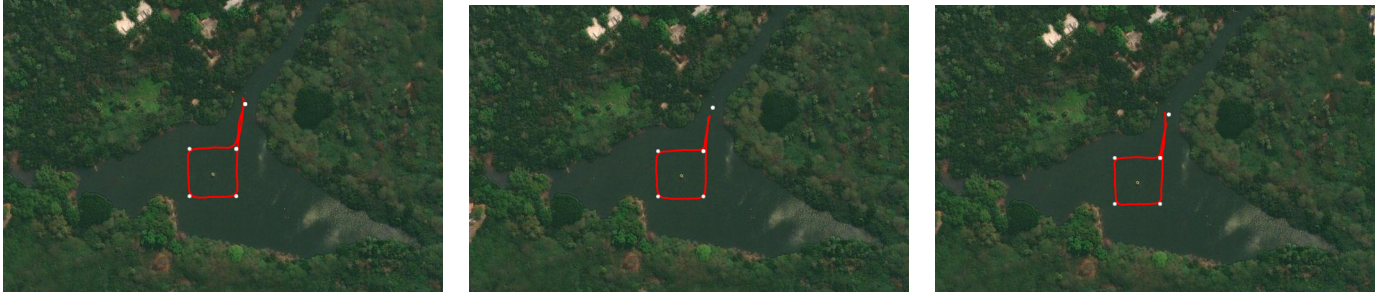
Fig. 2. Model scale square path experiments for DQN 3, DQN 5, and PPO from left to right. White markers denote the prescribed waypoints and the red curve denotes the measured vessel trajectory.
