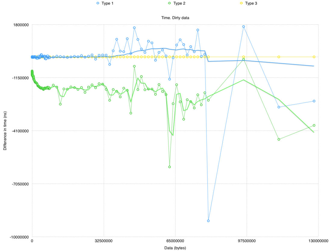
Figure 7.3: Performance of three ways of scheduling threads, Xeon 5130
