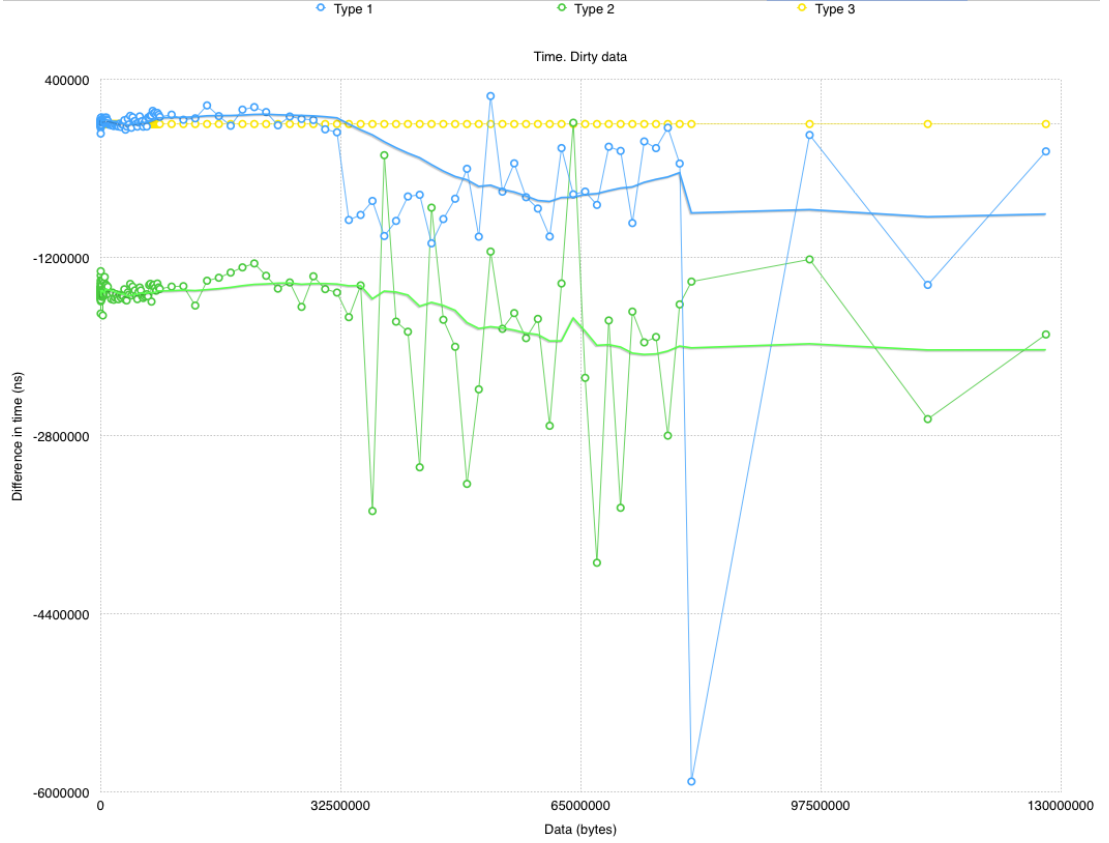
Figure 7.4: Performance of three ways of scheduling threads, Xeon E5-2695 v2
