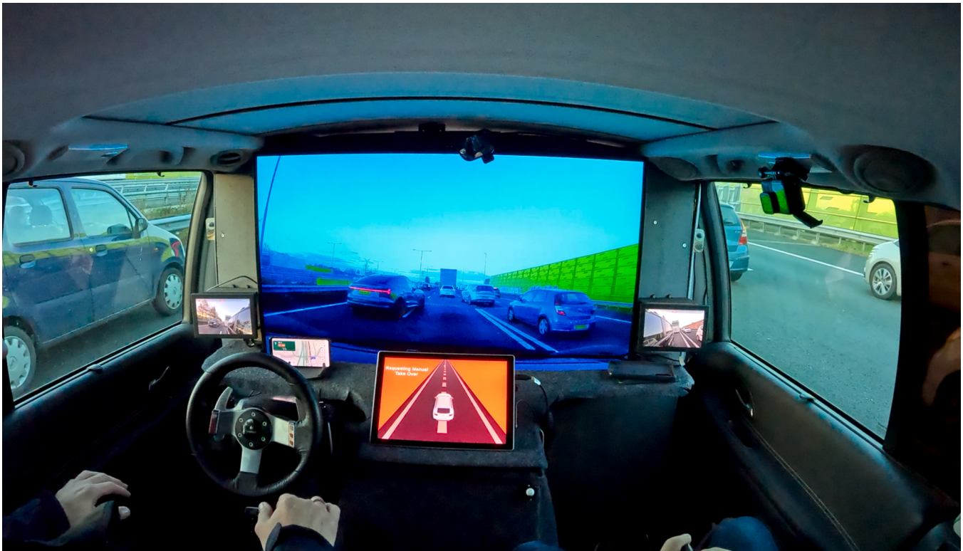
Fig. 2. The Wizard-of-Oz setup. The figure shows an urgent take-over request (TOR).
