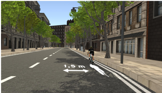
Road markings: Markings proposed by the Danish Cyclist Association to inform drivers of the 1.5-metre minimum overtaking distance rule[51].
