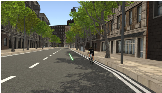
Car projection: A system that provides the driver with visual cues to indicate the appropriate distance for overtaking [2, 54].
