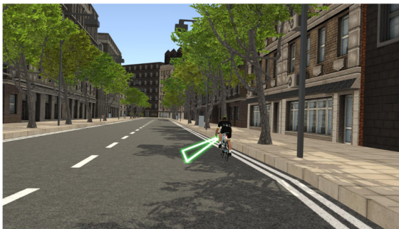
Laser projection: A system mounted on the bicycle handlebar that projects the safe passing distance from the bicycle onto the road similar to a solution used in London, UK [24, 54].
