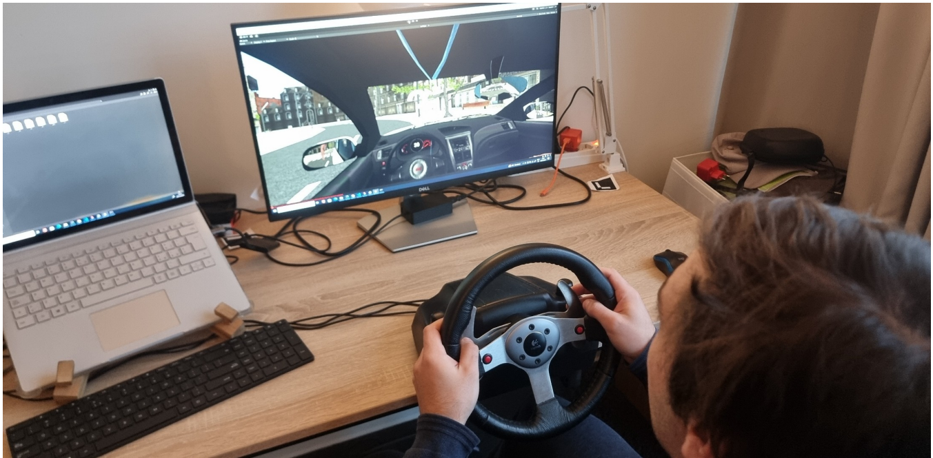
Figure 5: Experimental setup used during the laboratory experiment. Participants controlled a vehicle using a gaming steering wheel and paddles for speed adjustments with the simulation on a monitor.
