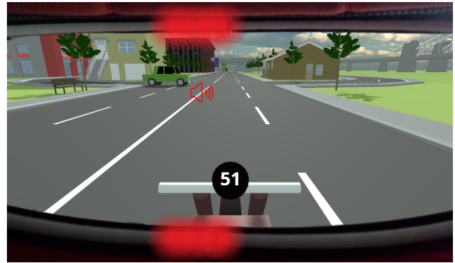
Figure 2: First-person rider perspective within the simulator. Multimodal feedback cues (peripheral visual illumination and spatial audio indicator) are overlaid to illustrate how a hazard event is presented to the participant. The number 51 is the current velocity (km/h).
