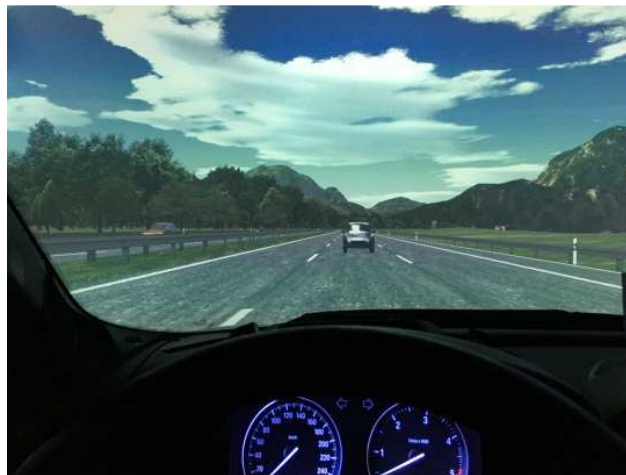
Figure 2. A take-over scenario. Participants could avoid the stationary car by steering left or right (Petermeijer et al., 2017a; Experiment 1).
