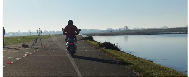
Figure 2 View from the inside of the car while following the scooter. Marks are made on the road using cones and tape. The measurements were conducted on a wind-free day (Measurement Series 2).
