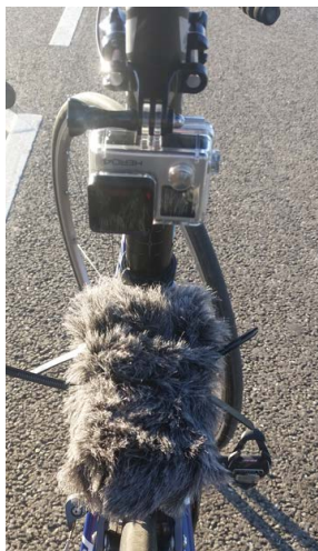
Figure 3 The smartphone with wind cover and GoPro camera mounted above the rear wheel of the bicycle (Measurement Series 3).
