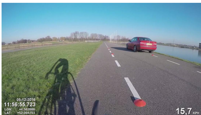
Figure 5 Screenshot of a video, with the car passing the moving cyclist. In this scenario, the smartphone, camera, and GPS tracker were mounted on the bicycle (Measurement Series 3).
