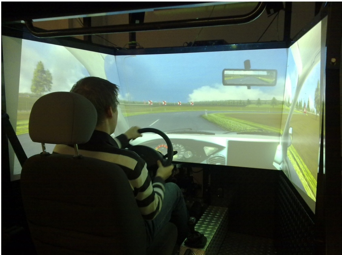
Figure 1. The driving simulator used in this research. In all trials, the visual projection was shut down.
