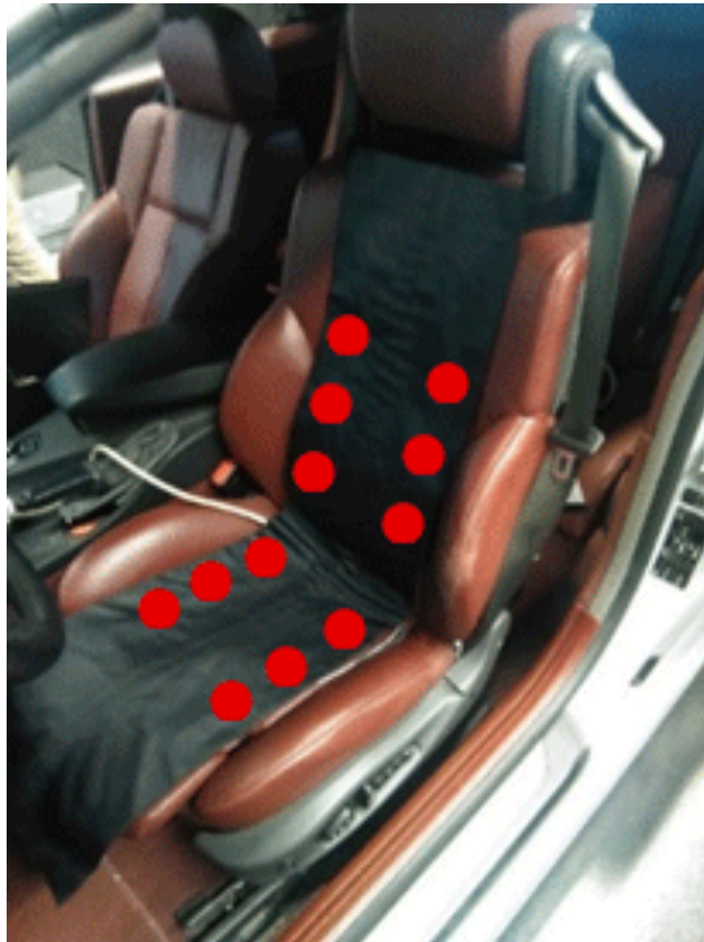
Figure 2. Vibration mat on the driver seat of the simulator. Red circles indicate the approximate locations of the vibration motors.
