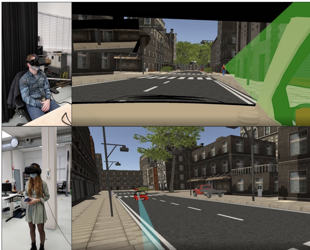
Figure 2: Laser visualizing eye contact between AV passenger (top) and pedestrian (bottom) in coupled simulator [17].
