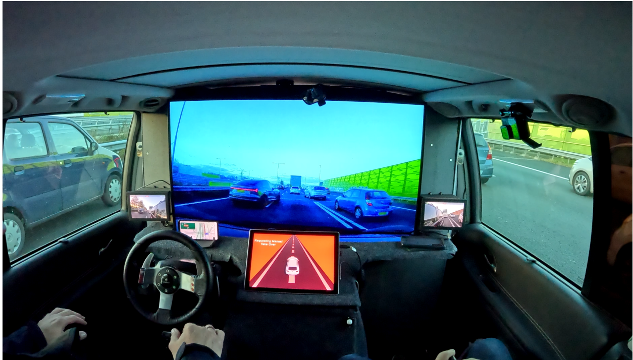
Figure 2. The Wizard of Oz (WoZ) setup. The figure shows an urgent take-over request (TOR).
