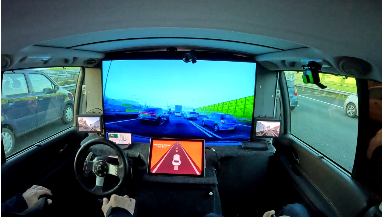
Figure 2. The Wizard-of-Oz setup. The figure shows an urgent take-over request (TOR).
