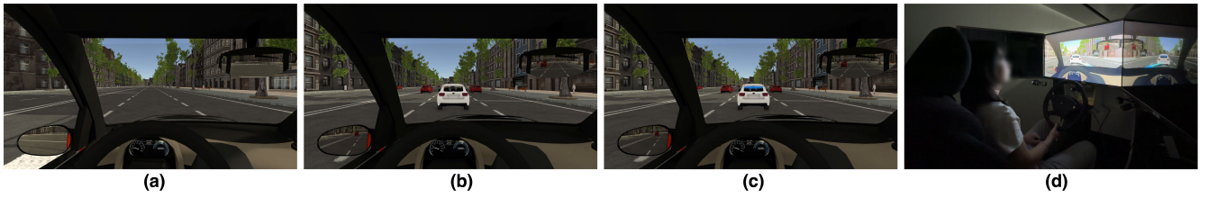
Figure 2: Video-based driving simulator scenarios and setup: (a) participant's view; (b) an MDV without a blue overlay; (c) an AV marked with a blue overlay; (d) a participant seated in the simulator cabin, interacting with the steering wheel HMI while viewing the scene on the front screen.
