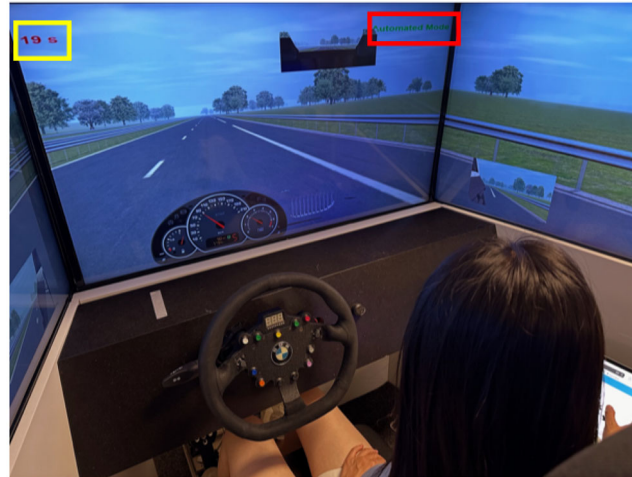
Figure 3. The current driving mode is shown in the upper right corner (red box), and the countdown time is shown in the upper left corner (yellow box).
