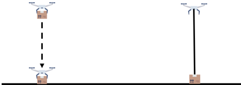
Figure 3: The two delivery methods, namely Land (left) and Cable (right).
