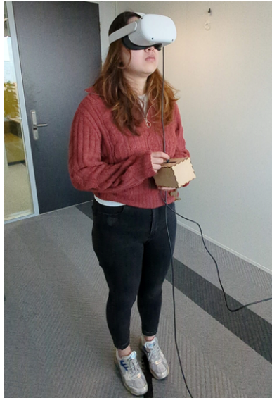
Figure 1: Participant with a head-mounted display in the VR experiment to assess feelings of uncertainty as a drone is flying towards her (in a straight line, curved line and either landing or doing a cable drop). In her hands, the participant holds a physical slider to express her uncertainty on a scale between 0 (no uncertainty) to 100 (absolute uncertainty).
