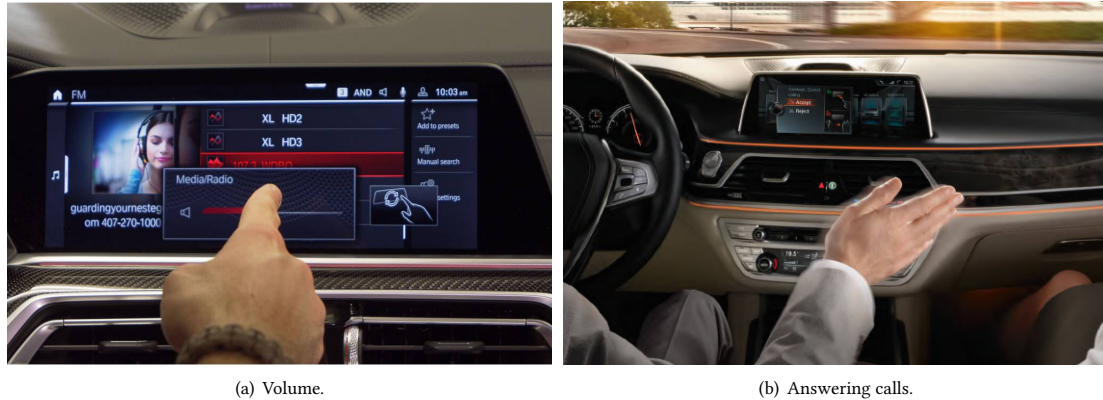
Fig. 2. Information pop-up indicating gesture controls are available for different functions in the 2015 BMW 7-series [11, 12].
