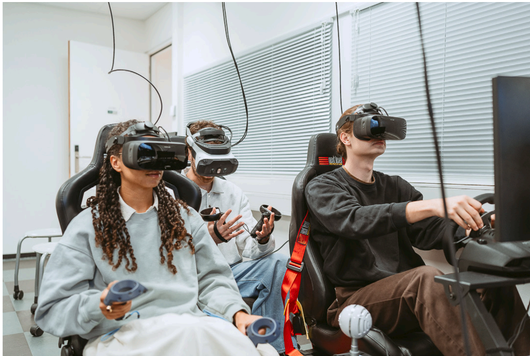
Fig. 3. Lab setup used in the study, showing VR headsets, seating arrangement, and driving hardware used during the simulation.
