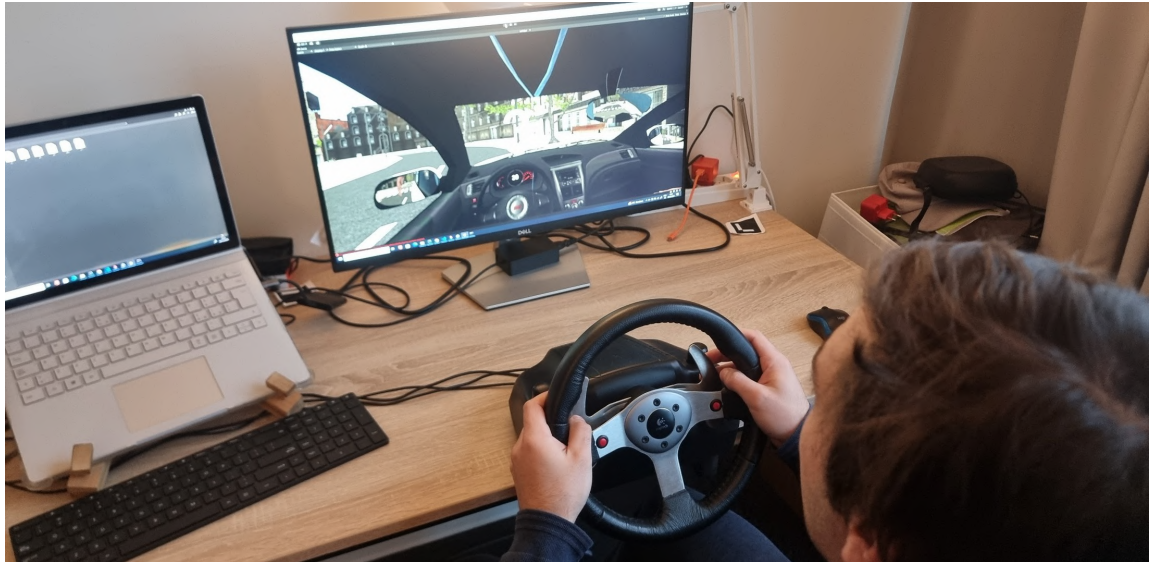
Fig. 5. Experimental setup used during the laboratory experiment. Participants controlled a vehicle using a gaming steering wheel and paddles for speed adjustments with the simulation on a monitor.
