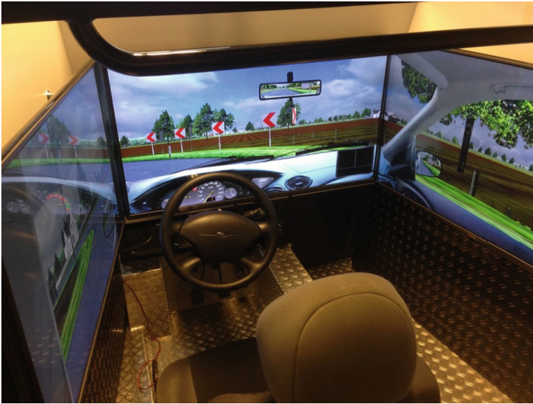
Fig. 1. The driving simulator used in this research. In all trials, the screens were turned off and participants wore headphones.
