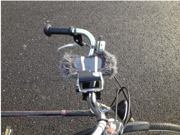
Fig. 6: Setup of experiment 4. The smartphone with windscreen mounted on the left side of the handlebar. The vertical axis of the smartphone parallel to the road. The camera mounted on the right side of the handlebar, to capture passing vehicles on film.
