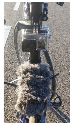
Fig. 5: Setup of experiment 2. The smartphone with windscreen cover and GoPro camera mounted above the rear wheel of the bicycle.
