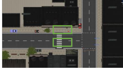
Fig. 6. Zoomed view of Environments 1 (left) and 2 (right), with box colliders in light green. These boxes are used to activated the right or left eHMI when there is driven through them.
