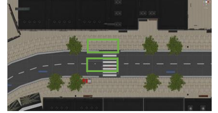
Fig. 6. Zoomed view of Environments 1 (left) and 2 (right), with box colliders in light green. These boxes are used to activated the right or left eHMI when there is driven through them.
