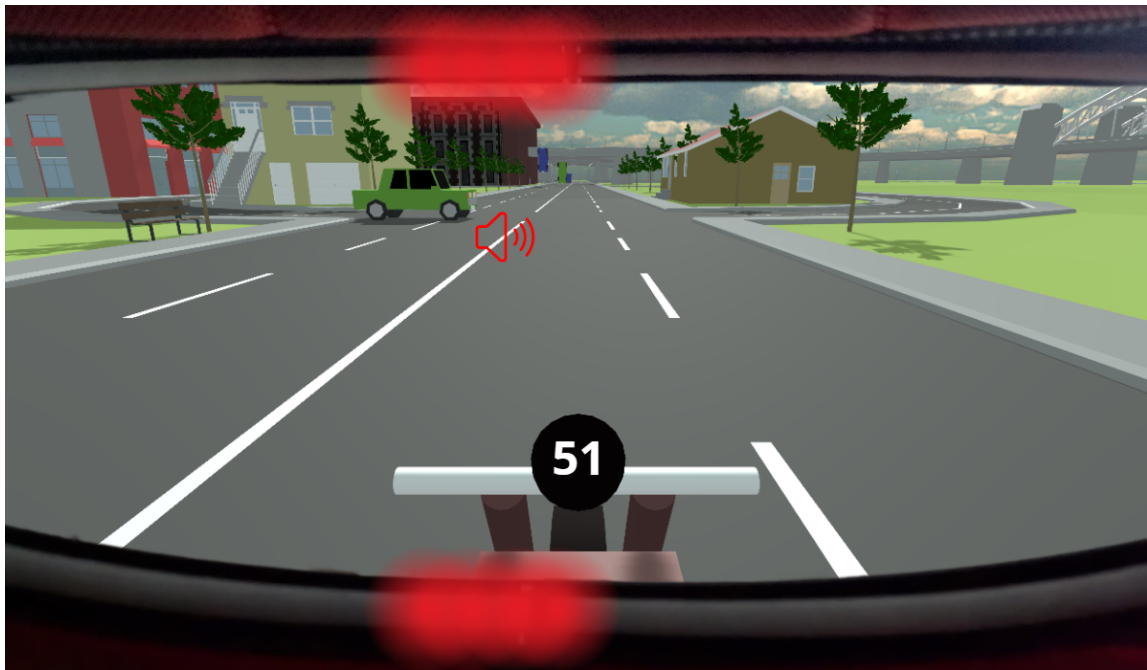
Fig. 2. First-person rider perspective within the Unity-based simulator. Multimodal feedback cues (peripheral visual illumination and spatial audio indicator) are overlaid to illustrate how a hazard event is presented to the participant. The speedometer displays the current velocity (51 km/h).
